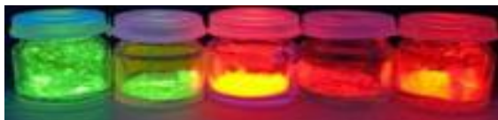
Fig. 1. Europium(III) and terbium(III) complexes under 365 nm UV light from left to right: Tb(tdh) 3 bpy, Tb(tmh) 3 bpy, Eu(tta) 3 bpy, Eu(tmh) 3 bpy and Eu(tdh) 3 bpy.
