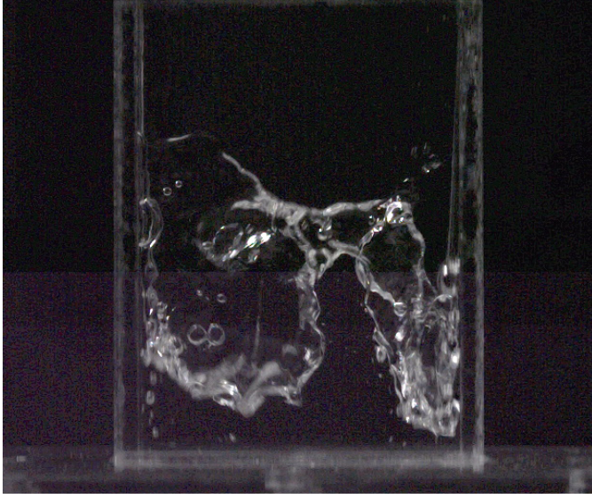
Fig. 1. Picture of isopropanol Faraday wave in a rectangular tank of dimensions L = 70 mm and l = 15 mm filled at h = (32 \pm 2) mm.
