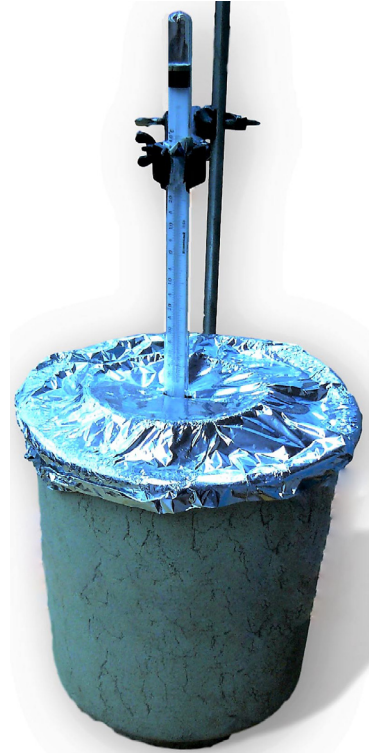
Fig. 6. View of the experimental system. Its properties are as follows. Inner pot: height – 15 cm, diameter – 9 cm, thickness – 6 mm. Outer pot: height – 40 cm, diameter – 18 cm, thickness – 6 mm. We used 10 kg of sand and 0.8 L of water.
