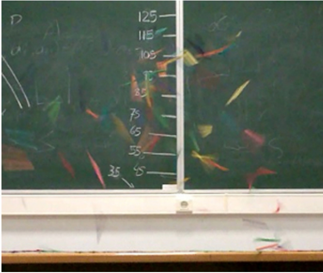
Fig. 2. The first experimental setup for measuring the maximum height of the popsicle stick cobras. The calibrated ruler is shown on the blackboard. This photo is a frame taken from the video that was capturing the popsicle explosion.
