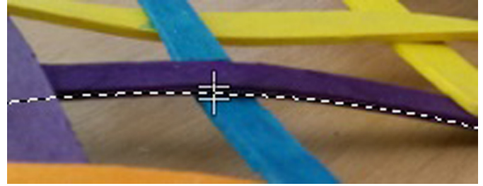
Fig. 3. A demonstration of the method for measuring the radius of curvature. A dashed circle is fitted alongside the bent stick.
